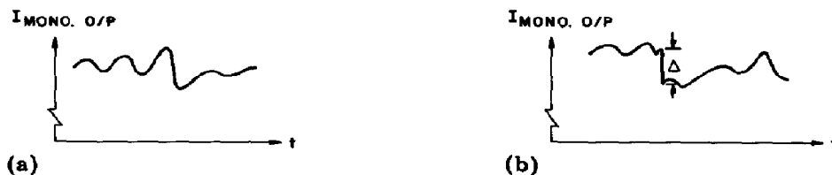
Fig. 1. (a) Monochromator output without concentration modulation; the absorption is masked by the fluctuation and drift of the light source. (b) Monochromator output with concentration modulation; the modulated step change \Delta is detectable from the noise.
